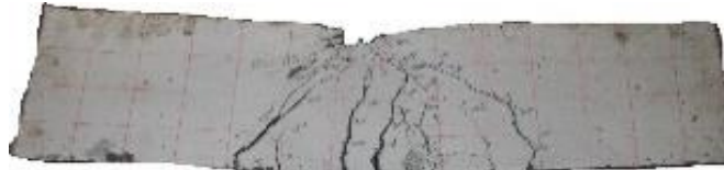
a) T=38^{\circ}\text{C} (flexural failure)
