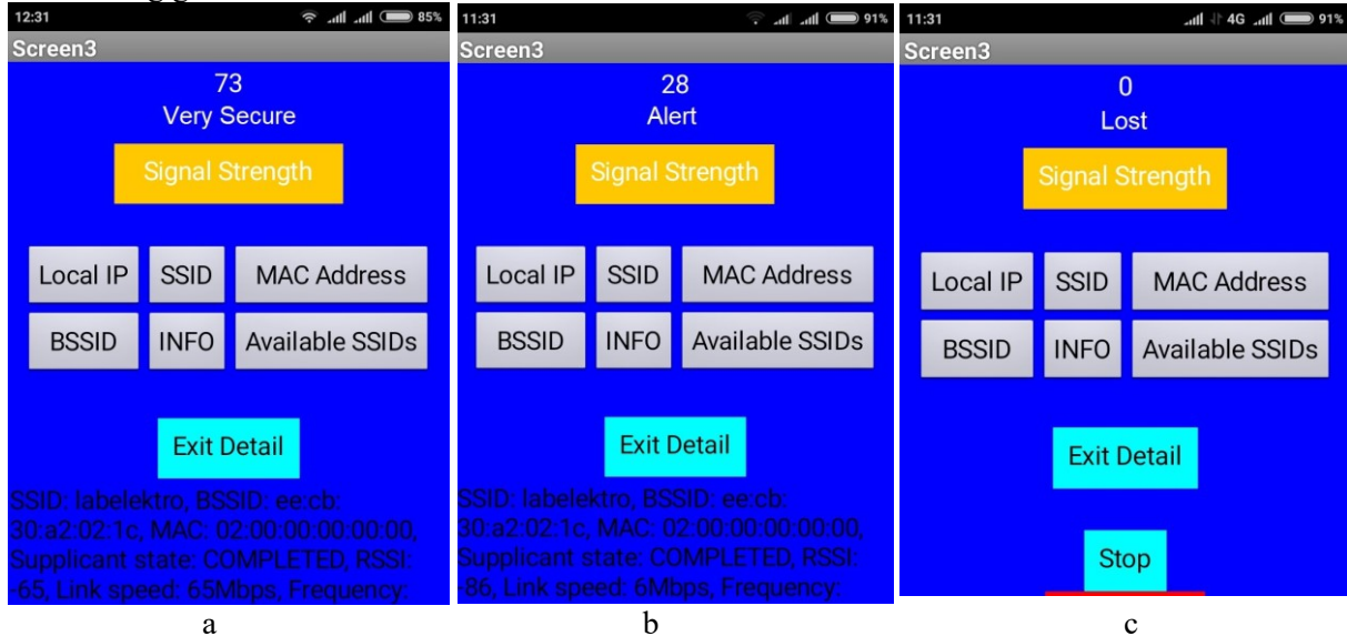
Figure 5. a. Display of membership Fuzzy Very Secure membership with RSSI -65 dBm b. Fuzzy Alert membership display with RSSI -86 dBm c. The membership display of Fuzzy Lost with RSSI is smaller than -90 dBm
