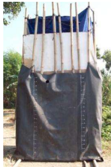
Figure 2. Pontoon with bamboo materials modeled in this research[10]
