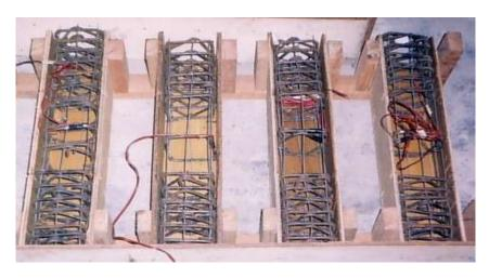
Figure 3 Typical reinforcement cages for confined concrete.
