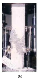
Figure 6 Failure of specimens: (a) tie spacing 50 mm, (b) tie spacing 100 mm.
