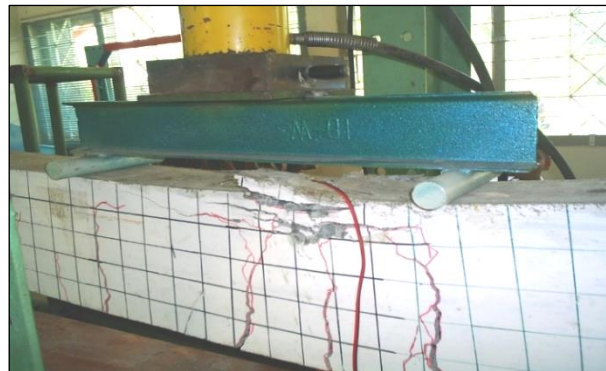
Figure 11. Normal beam failure under two points loads
