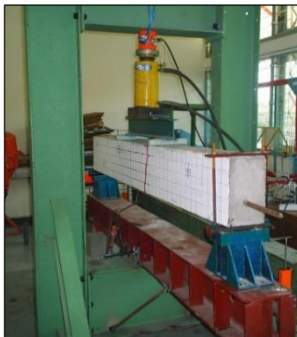
Figure 9. Experimental set-up for the normal beam and beam with CFRP
