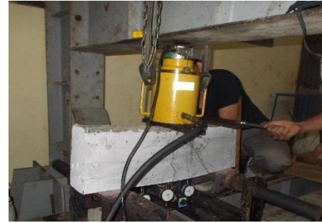
Fig. 4 Testing the beam to collapse
