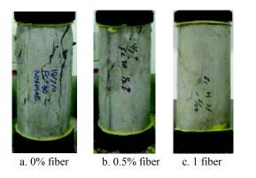
Figure 3. Cracking of cylinder specimens under compressive loading
