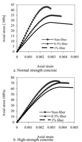
Figure 4. Stress-strain curves under compressive loading It is clear from Figure 4 that the shape of the stressstrain curve up to maximum stress for both normal and high-strength concrete without Gunny Sack fiber, has a steeper slope and is more nearly linear and the explosive manner in the post peak. For fiber concrete with added Gunny Sack shows that the descending branch are more ductile.
