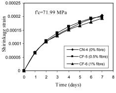
b. High strength concrete Figure 7. Shrinkage behaviour
