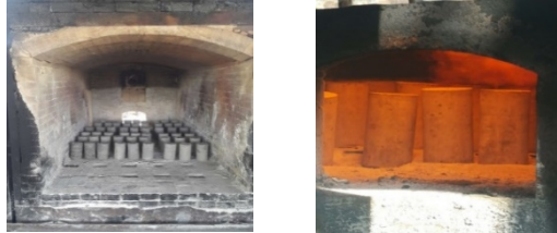
Fig.2 The process of preparation and burning of test specimens
