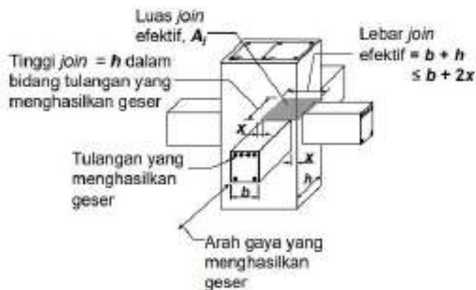
Gambar 12.19. Area efektif join, A_j
