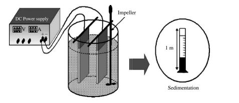
Figure 1 Static system apparatus
