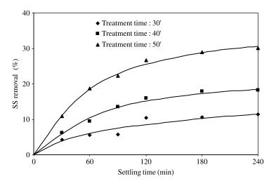
Figure 5 TSS removal efficiencies as a function of settling time (l = 0.8 A; t = 30 - 50 min)
