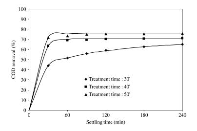
Figure 6 COD removal efficiencies as a function of settling time (l = 0.8 A; t = 30-50 min)
