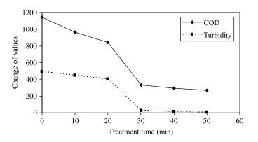
Figure 3 Effect of treatment time on the removal of COD and Turbidity (I = 0.8 A)
