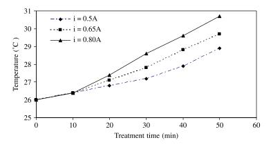
Figure 4 Effect of treatment time on temperature
