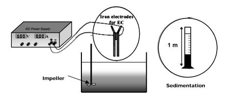
Figure 2: Static system setup of electrocoagulation process
