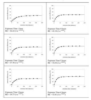
Figure 2 Removal percentage of suspended solids by circulation flowing method using magnetic field of 0.55 T at 2 mL/s flow rate with varying exposure times of 1–6 h
