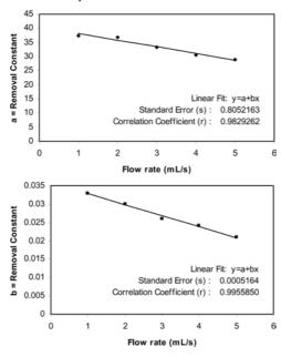
Figure 6 The effect of flow rate on the removal constant of suspended solids in magnetic force of 0.55 T at 6 h treatment period
