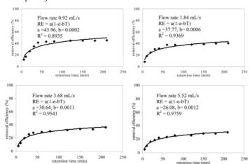
**Figure 8** The comparison removal efficiencies of suspended solids by circulation flowing method using magnetic field of 0.55 T at 2 h treatment period, with verified flow rate and without pH adjustment
