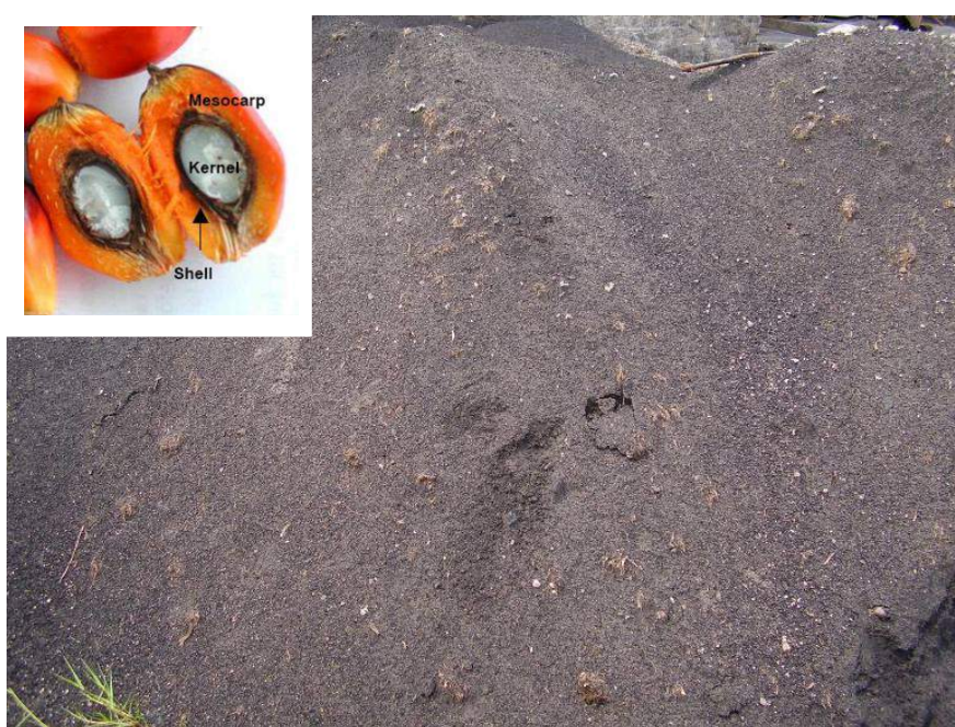
Figure 2.1 - Oil Palm Fruit Ash after burning (inside is fruitlet of palm oil fruit)
