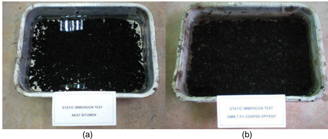
Figure 3.5 - Static-immersion test of base bitumen (a) and 7.5% C-OPFA-MB (b) (after 48 hours)
