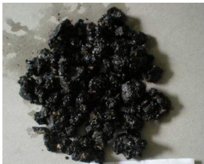
Figure 4. Boiling water test result of SMA-14 mixture
